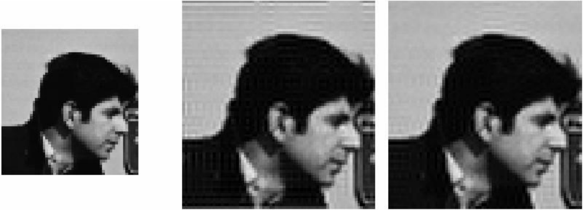
Figure 1. Comparison of image scaling algorithms. Left: the original image. Middle: the scaled image computed using DFT-domain convolution ( \sigma = \sqrt{2} ). Right: the scaled image computed using DCT-domain convolution ( \sigma = \sqrt{2} ).
