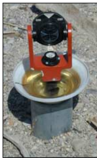
Figure 5.5 - the reflector placed on one of the pipes.
