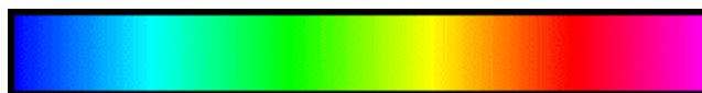
Figure 5.7 – One cycle (fringe) of colors, standing for one cycle of the phase change ( 2\pi ).
